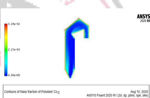
Fig. 36 CO2 mass fraction in Case 8
