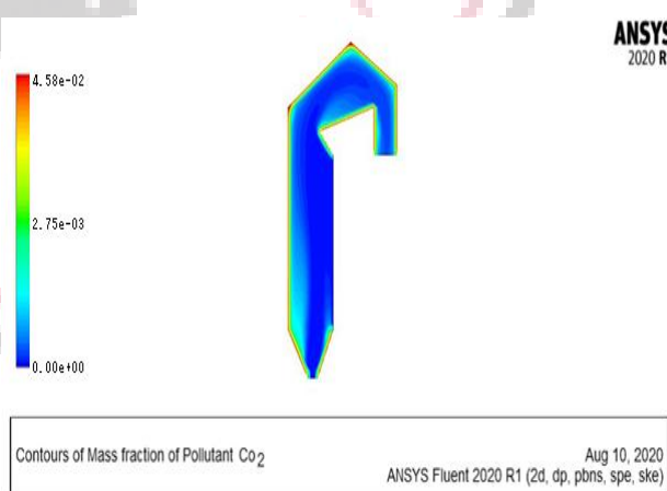
Fig. 32 CO2 mass fraction in Case 4
